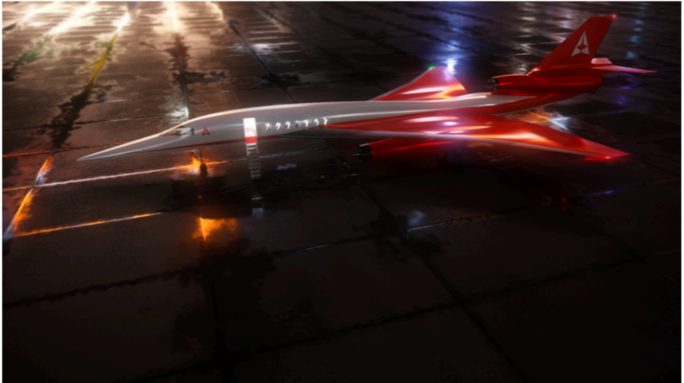
The Aerion AS2 will offer boomless cruise up to Mach 1.2, and a max cruise speed of Mach 1.4 Aerion Supersonic
